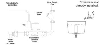
Turn off the water supply & identify a suitable location for the valve. Remove a section of pipe & fit the valve taking note of water flow direction marked on the underside of the valve with either an "IN" mark or 1 for "In" & 2 for "Out".
