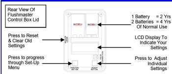
Insert the batteries then immediately press the reset button & wait 5 seconds for the LCD display to illuminate.
