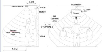
The Flushmaster will ideally be located on the ceiling in the centre of the urinals to be controlled, facing downward & at approx 0.5m - 0.8m from the cistern wall.
