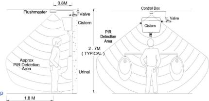
Avoid if possible locating the control box near heat sources (e.g. radiators), or where sunlight can fall on the PIR detector window.
