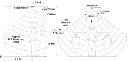
Avoid if possible locating the control box near heat sources (e.g. radiators), or where sunlight can fall on the PIR detector window.
